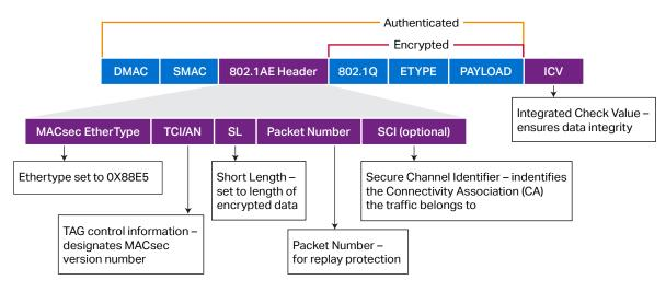
Figure 2. MACsec authenticated and encrypted frame and MACsec frame format
