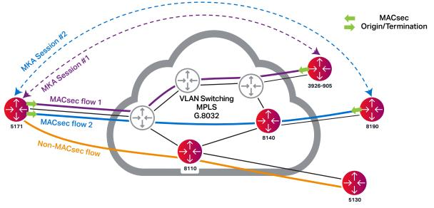
Figure 5. Ciena's end-to-end MACsec allows MACsec to encrypt the payload but still transmit data across intermediate network VLAN tags, MPLS labels, or SR labels in the clear
