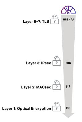
Figure 1. Encryption techniques across OSI layers and their performance
