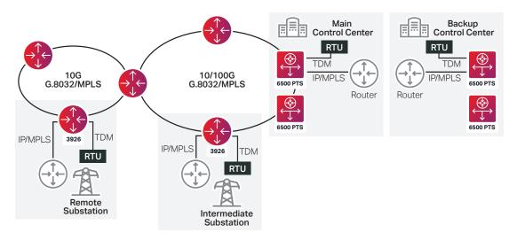
Figure 2. IO utility TDM network
