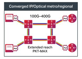
For metro Reconfigurable Optical Add/Drop Multiplexer (ROADM) networks, WL5n Universal CFP2-DCO supports Optical Transport Network (OTN) modes for both ITU-T/FlexO and Open ROADM MSA-based interoperability as well as performance-enhanced OTN-MAX modes for maximum reach from a CFP2-DCO form factor.
